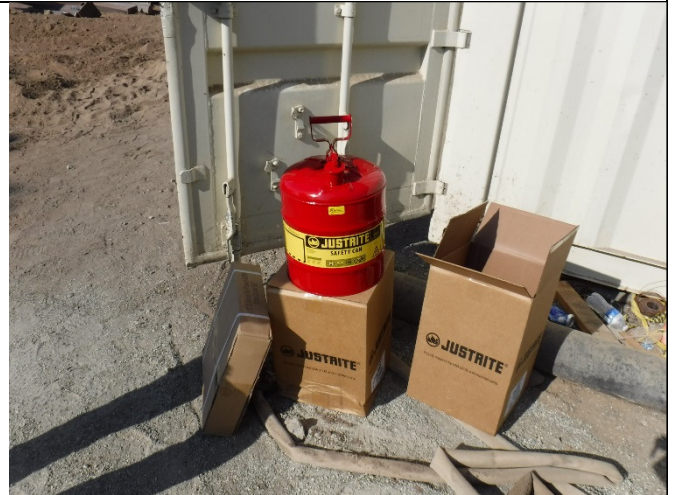
Photograph 4. Proper fuel containers were observed onsite. All plastic fuel containers were being removed from this job site.
