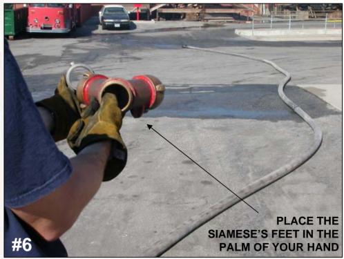
Once you've determined which line to tap into, pick up the siamese and face the nozzle (fire). Position the male end of the siamese facing toward you (with the siamese's feet in the palm of your hand) and the two female ends of the siamese facing away from you. Choose the left female coupling of the siamese and connect that coupling to your double male fitting and then to the hose. This step will ensure you connect the correct side of the siamese to the hose. (Photo #6)
